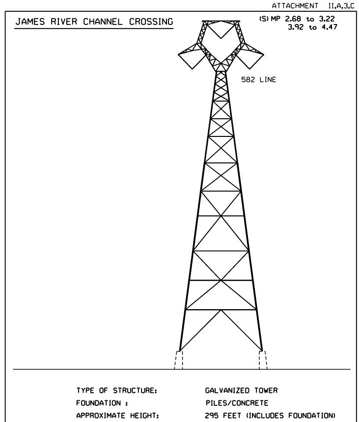
APPROXIMATE HEIGHT: AVERAGE SPAN LENGTH: CONDUCTOR TYPE: RIGHT OF WAY WIDTH: APPROXIMATE LENGTH: PILES/CONCRETE 295 FEET (INCLUDES FOUNDATION) 1200 FEET ALUMINUM BY PERMIT 1.09 MILES
