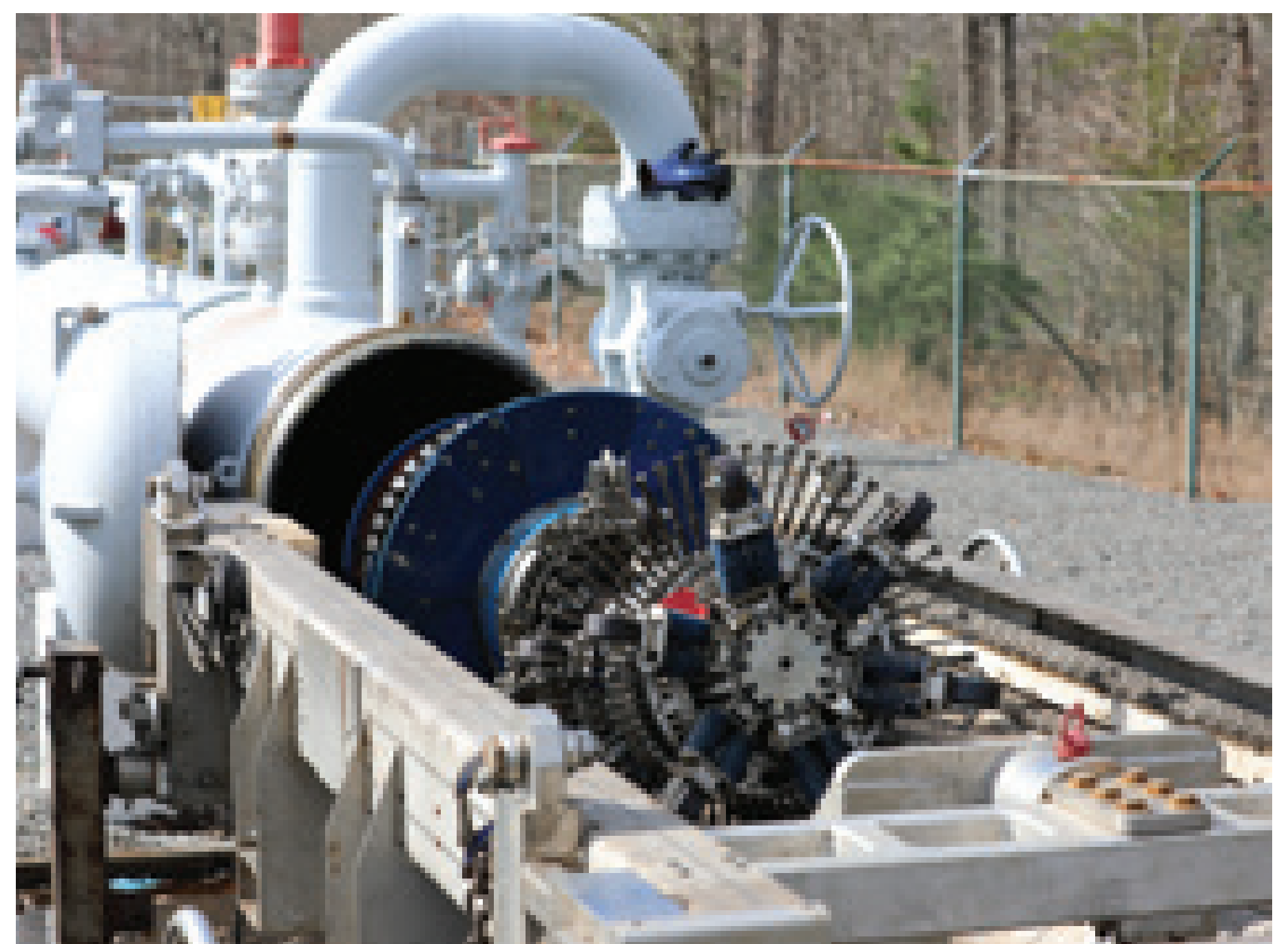
Although pipelines operate underground, in-line inspections can be conducted using smart pigs.
