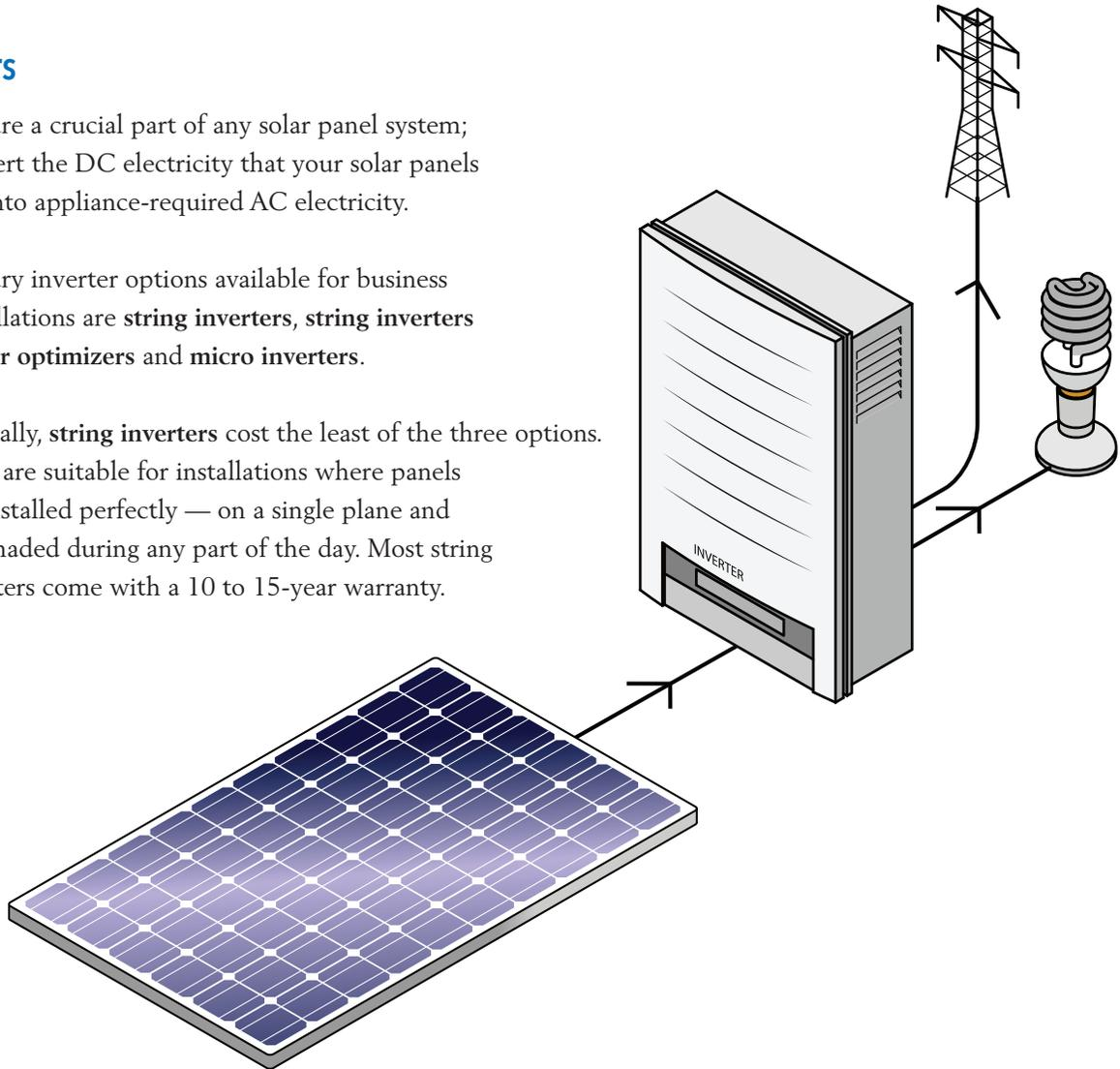
**String inverters with power optimizers and micro inverters** are more expensive, but are suitable for installations where one or more panels may be shaded, or where panels are installed on multiple planes and/or facing different directions. They also allow you to monitor the power production of each individual panel. Generally, warranties are 10 to 15 years for string inverters with power optimizers and 25 years for microinverters.
