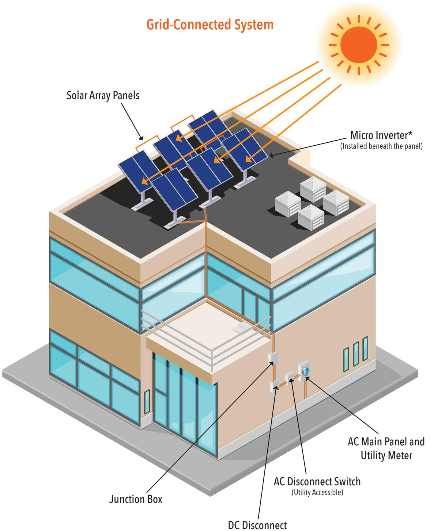
*\*Note: Other inverter types include string inverters and string inverters with power optimizers. See pg. 7 for details.*
