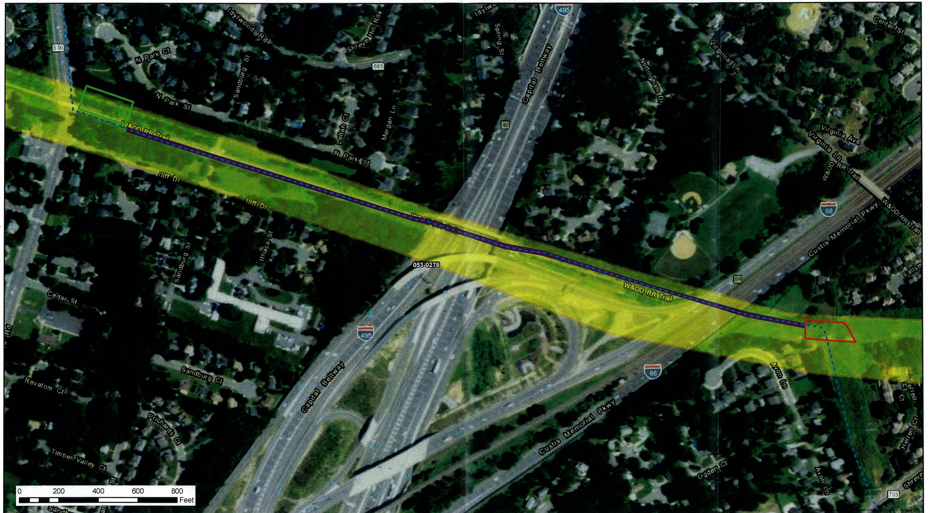
Figure 3.7.1-1 Locations of HDD versus open-trench construction segments along 053-0276 for Underground Alternative 05 Idylwood-Tysons 230 kV Underground Transmission Line Project Fairfax County, Virginia ERM C:\Users\vincent.mace\Documents\ldlewood 7-17\Underground Lines\ldlewood Underground Tree Removal sheet 11-1.mxd | REVISED: 11/01/2017 | SCALE: 1:3,500 Dominion Energy DRAWN BY: GIS
